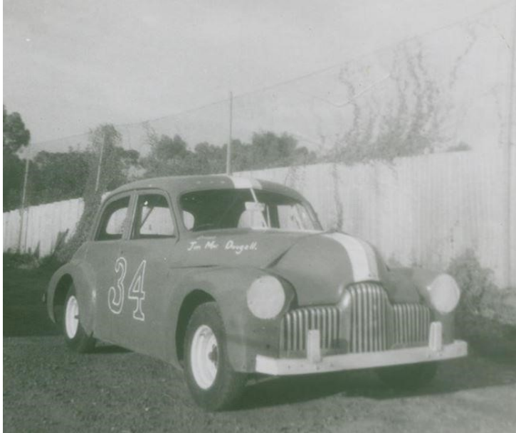
1969—Jim's '1948 FX Stock Car No. 34' complete with roll bars, wide wheels, reinforced front bumper & monogrammed bonnet.
